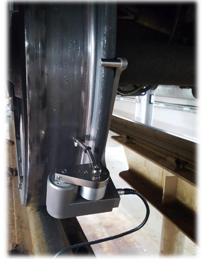
Wheel profile measured using a miniprof
